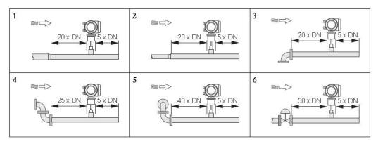
1 = Reduction, 2 = Expansion, 3 =  $90^{\circ}$  elbow or T-piece, 4 =  $2 \times 90^{\circ}$  elbow, 5 =  $2 \times 90^{\circ}$  elbow (3-dimensional), 6 = Control valve or pressure regulator.
