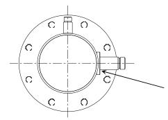
Before Welding, the base should be processed as the same as the circular arc of pipe to ensure sealing
